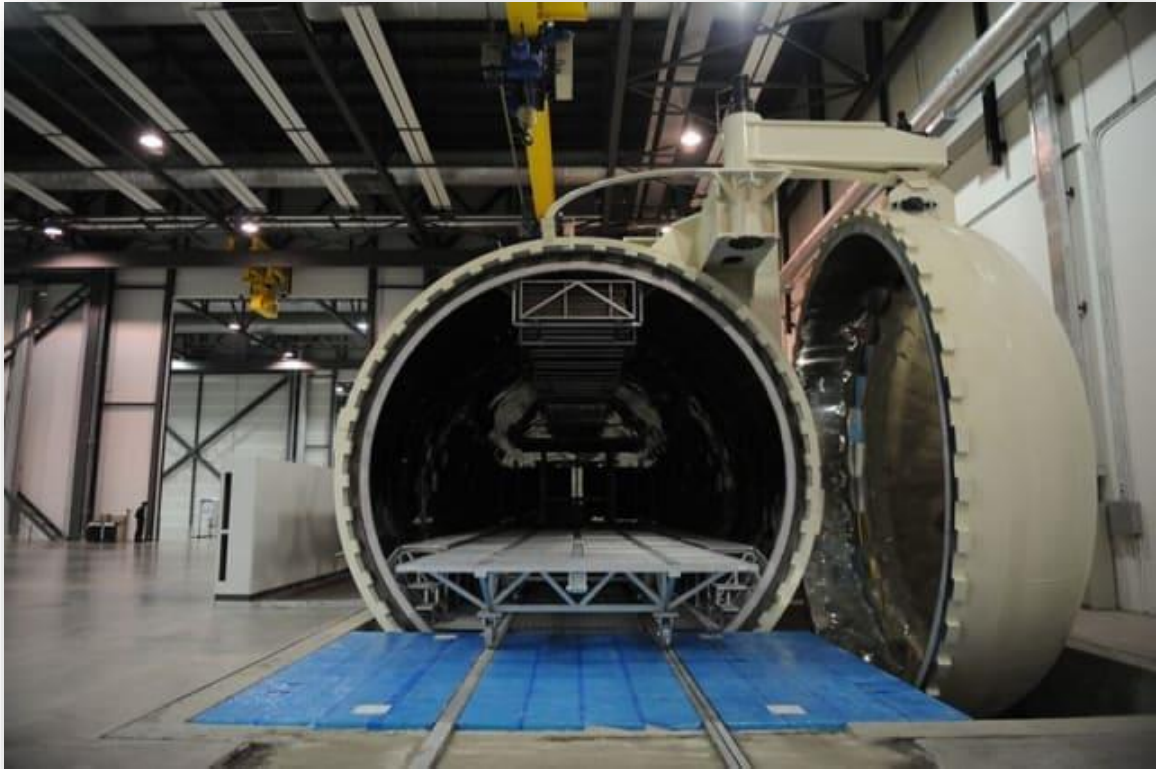
Large autoclaves are essential in large scale composite manufacturing
