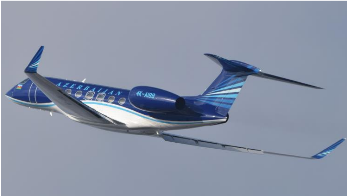
The Gulfstream G650's tail rudder and elevators are made of carbon fiber/polyphenylene sulfide (PPS) thermoplastic composite.
