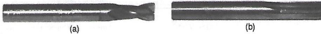
Fig. 17 a Two-flute helical end mill (helix angle; 30°, rake angle; 10°/30°, clearance angle; 9°), b Six-flute straight /0° helix angle end mill (Davim and Reis 2005)
