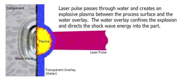
Creates a compressive bi-axial state of stress in the material
