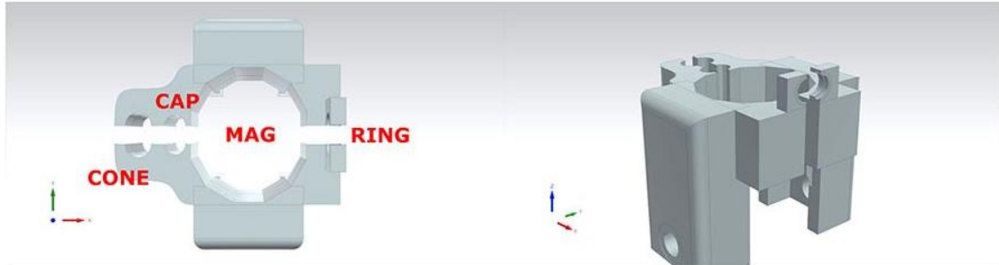
The gripper fingers were designed to perform multiple tasks. The left images shows a top-down perspective, highlighting the central decagonal hole for gripping the magazine. The right image shows the hole for the cap and a conical hole for gripping the cone. Source:
